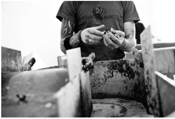
Iraq War veteran Eli Wright feeds the Hollander beater with snippets of combat uniforms (50% cotton, 50% nylon) in the Hollander beater. Combat uniforms range in patterns and colors. Some soldiers had dark forest camouflage, which explains the deep value of this slurry. Towards the end of the beating cycle, veterans add war paraphernalia such as bandannas worn to cover their faces during dust storms and Iraqi paper money.
